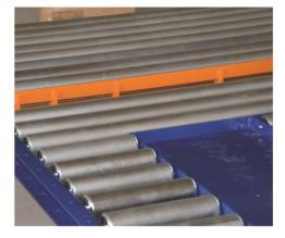
The RLP family of gravity roller conveyors are used at the beginning or end of gravity or powered lines for loading or removing pallets or large boxes. The end part of the conveyor is fork-like to enable a hand-pallet to enter the loading area to deposit or remove pallets. They are virtually maintenance-free and are manually operated thus require no energy.
